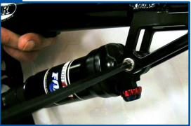
**O8** Place the shock in a soft-jawed vice being careful not to crush any shock parts. Place the breaker bar through the body eyelet and attempt to pull out the body shaft. If you cannot pull it out, this confirms that the shock is "stuck down." Proceed with caution.
