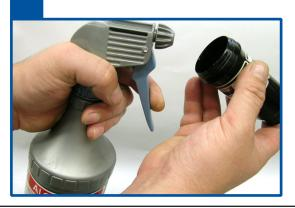
Although a full set of replacement seals has been provided, it is not necessary to replace all of them on a brand-new unused shock. The body seal (quad ring), however, still needs to be replaced, as shown in steps 17-18.
