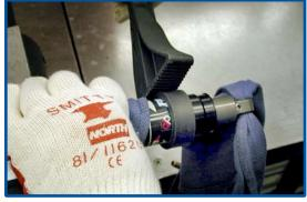
Remove the shop towel from the body eyelet then fully remove the air sleeve.
