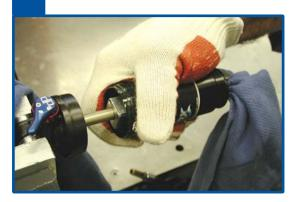
Clean the inside of the air sleeve with isopropyl alcohol or parts cleaner.
