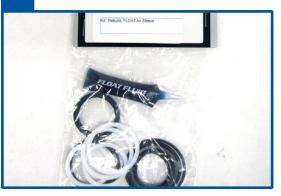
16 Two shaft eyelet o-rings are supplied with the Air Sleeve Rebuild Kit; a 2000-04 FLOAT rear shock uses the thicker o-ring, the 2005 and newer uses the thinner o-ring.
