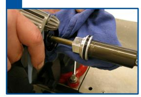
15 When replacing the air sleeve wiper, seal and backup rings, ensure that they are properly oriented. Lightly lubricate all seals and rings before installing them. Use no more than half of the FLOAT Fluid pillow pack for this entire procedure.
