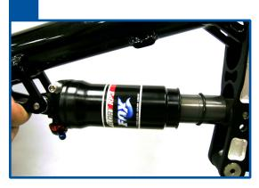
Remove reducers from the body end of the shock using a 3/8" bolt extractor.
