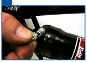
Remove the mounting hardware and remove the shock from the bicycle. In most cases, a hex wrench is all that is necessary to remove the mounting hardware. Hex wrench size will vary depending on manufacturer.
