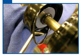
21 Replace the backup ring, seal, backup ring, and dust wiper into the air sleeve seal glands. Tip: Squeeze the backup ring like a "potato chip," as shown, to facilitate installation.
