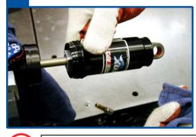
10 Finish unscrewing the air sleeve by hand and pull it back from the shaft.
