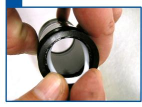
Place 2cc of FLOAT Fluid into the air sleeve. Do not screw the air sleeve on at this time.
